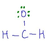
In this example, we could only put electrons on the oxygen atom, since the outer hydrogen atoms were "full" with two electrons.
