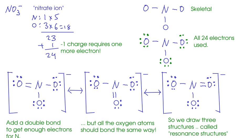
There's not really a double bond in the structure that bounces around. The real molecule has some electrons that are shared between all of these atoms - and this is just how we show delocalized bonds with Lewis structures.
