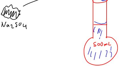
A VOLUMETRIC FLASK is a flask that is designed to precisely contain a certain volume of liquid.
