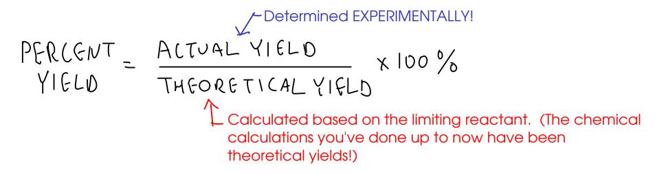
... the percent yield of a reaction can never be greater than 100% due to conservation of mass! If you determine that a percent yield is greater than 100%, then you've made a mistake somewhere - either in a calculation or in the experiment itself!
