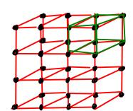
Here's a crystal lattice in three dimensions. This one is called a SIMPLE CUBIC lattice. This simple structure can be found in some solid metals like polonium. A polonium atom occupies each lattice point.
