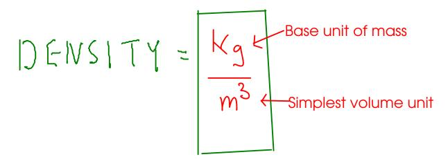
Both the kg and the cubic meter are too large for routine lab work! (Our balances have a maximum capacity of about 200 grams!)
