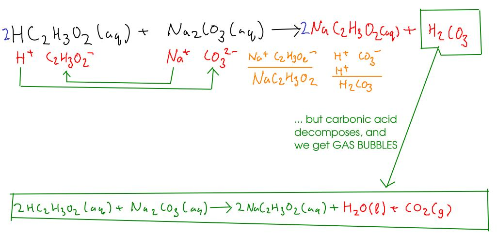
This is the overall process. We show carbon dioxide and water as products, since we want to show the reaction as it's actually observed -with carbonic acid broken down to water and (gaseous) carbon dioxide.
