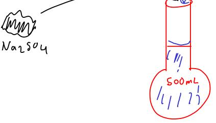
A VOLUMETRIC FLASK is a flask that is designed to precisely contain a certain volume of liquid.
