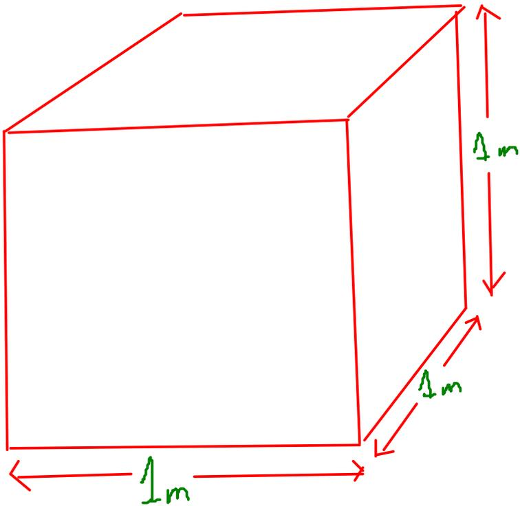
Problem: The cubic meter is a large unit ... too large for lab scale and medical work.
