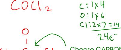
Choose CARBON as the central atom since it needed to gain more electrons (4) than either oxygen (2) or chlorine (1).
