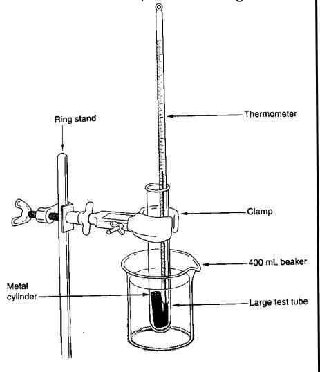
Then, we'll put the metal cylinder into a coffee-cup caporimeter and measure the temperature rise of the calorimeter's water:
