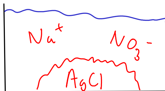
Insoluble \text{AgCl} falls out of solution as it is formed - "precipitation"
