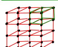
Here's a crystal lattice in three dimensions. This one is called a SIMPLE CUBIC lattice. This simple structure can be found in some solid metals like polonium. A polonium atom occupies each lattice point.
