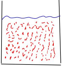
The reaction takes place only on the surface of the cube. Here, the reaction takes place on the surface area of each fragment. In total, this is a much LARGER surface than the cube.
