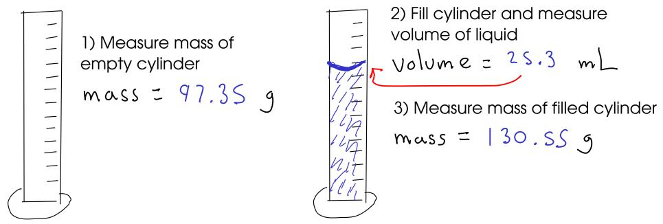
5) Density = mass liquid / volume liquid Density =  $\frac{33.20 \text{ g}}{25.3 \text{ mL}}$ =  $\left| .3 \right| \frac{9}{mL}$
