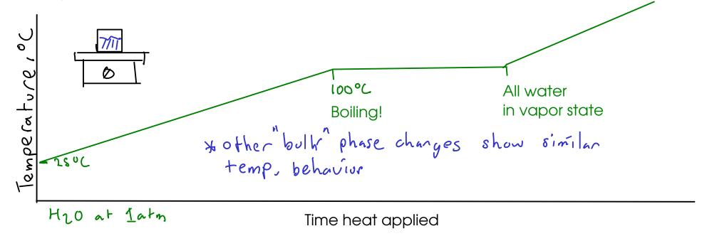
DURING THE BOILING PROCESS, as long as you have some liquid water remaining, the temperature will remain constant - EVEN AS YOU CONTINUE TO APPLY HEAT!
