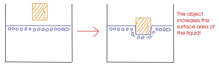
For the object to penetrate the liquid surface, it must push water molecules at the surface apart. Since these water molecules ARE ATTRACTED TO ONE ANOTHER, the liquid will resist!
