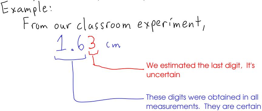
THIS MEASUREMENT HAS "THREE SIGNIFICANT FIGURES"!
