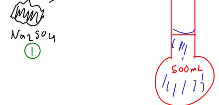
A VOLUMETRIC FLASK is a flask that is designed to precisely contain a certain volume of liquid.
