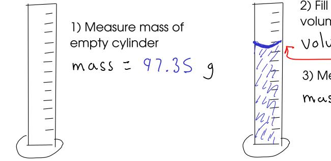
2) Fill cylinder and measure volume of liquid Volume = 25.3 m 3) Measure mass of filled cylinder mass = |30.55 g
