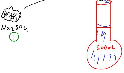
A VOLUMETRIC FLASK is a flask that is designed to precisely contain a certain volume of liquid.
