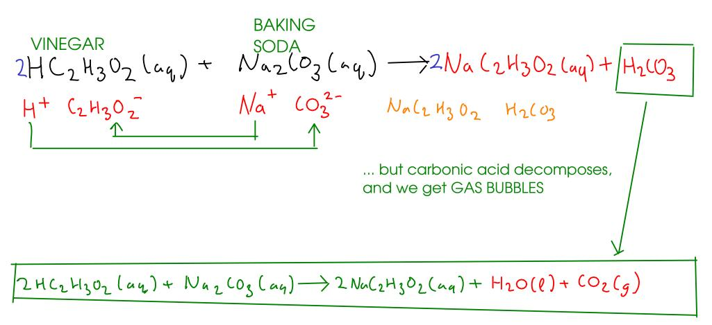
This is the overall process. We show carbon dioxide and water as products, since we want to show the reaction as it's actually observed -with carbonic acid broken down to water and (gaseous) carbon dioxide.
