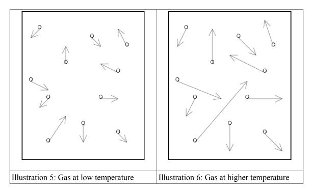
The length of the arrows in front of the gas molecules indicates the speed of the gas molecules. But what conclusions can we draw from all this? How can we relate this to the empirical gas laws?
