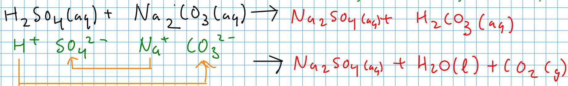
Driving force is the release of carbon dioxide gas!
