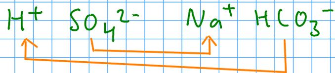
... but when we mix sulfuric acid and sodium bicarbonate, we observe BUBBLES. We need to write an equation that agrees with our observations. We know that carbonic acid decomposes, so we go ahead and put that into our equation.
