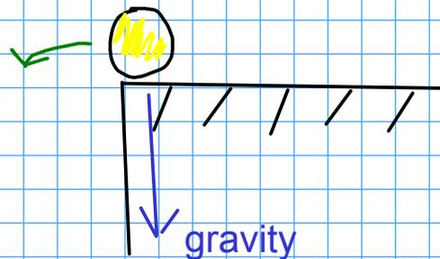
When the ball falls, its potential energy is converted to kinetic!
