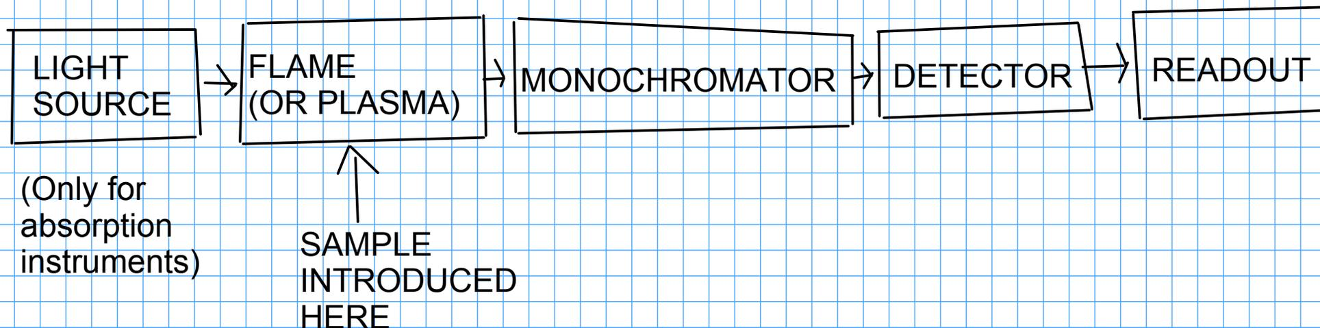
**SOURCE:** "hollow cathode lamp" - lamp whose cathode is made of the element(s) that we want to analyze. These atoms produce light of the desired wavelengths. This light is perfectly suited to use for the analysis.
