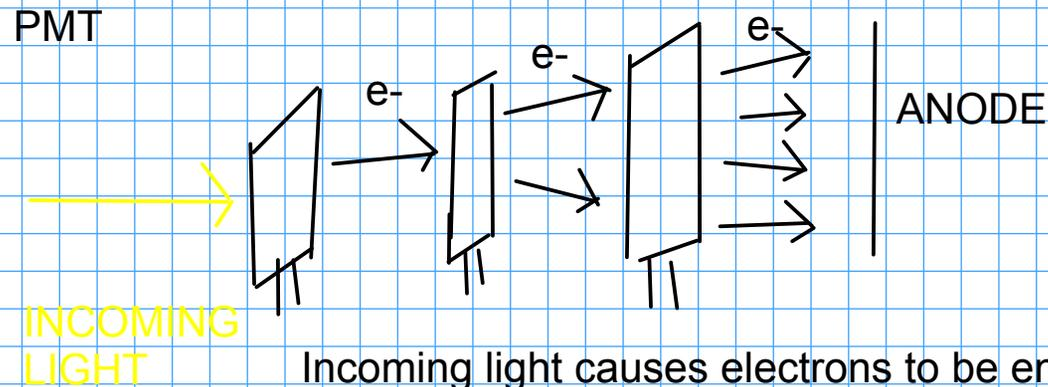
Incoming light causes electrons to be emitted from the cathode of the photomultiplier tube, leading to a cascade of electron emission in the tube, Each photon ends up causing the release of many electrons, giving the PMT high sensitivity!
